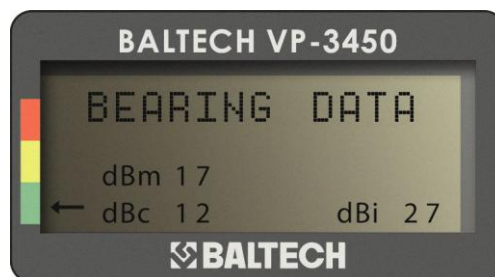
Figure 4-4. Shock pulse measurement.
