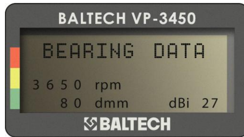
Figure 4-3. Setting rpm and diameter. Step 2.
