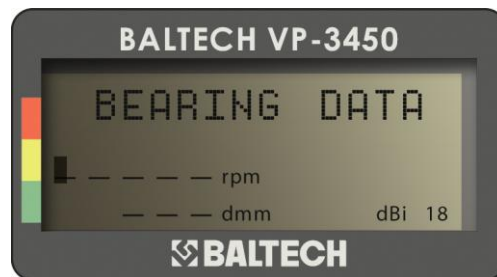
Figure 4-2. Setting rpm and diameter. Step 1.
