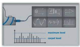
Total shock pulse intensity increases with decreasing of lubrication film thickness. Pronounced shock pulse peaks indicate bearing defects.
