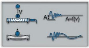
The shock pulse method can be illustrated by the example of a metal ball fall on a metal object. The shock waves will appear in both objects. The shock pulse amplitude is equal to the impact velocity function.
