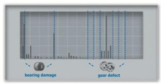
The bearing vibration monitoring allows detecting irregularities in equipment, and to define the reason of such irregularities the spectral vibration diagnostics should be used.
